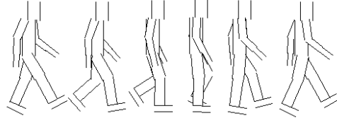
Fig. 2. Movement states of walking represented by the visible contours of the 3D model ( pose = 0.0, 0.1, 0.2, 0.3, 0.4, 0.5 )
