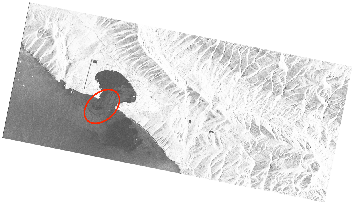
Figure 4: The orthorectified TerraSAR-X image showing the bay of Gelendzhik and the coastal area as well as the Black Sea. The brightness has been raised in order to ensure the visibility of the biogenic marine surface films' signatures near the bay area (marked red).
