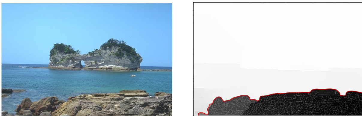
Figure 3.19: An example for the normalized cut approximation; the image on the right shows the entries for the second smallest eigenvector and the resulting cut (red line) after thresholding. The region adjacency graph has been derived from a watershed segmentation and has edge weights from colorMean .
