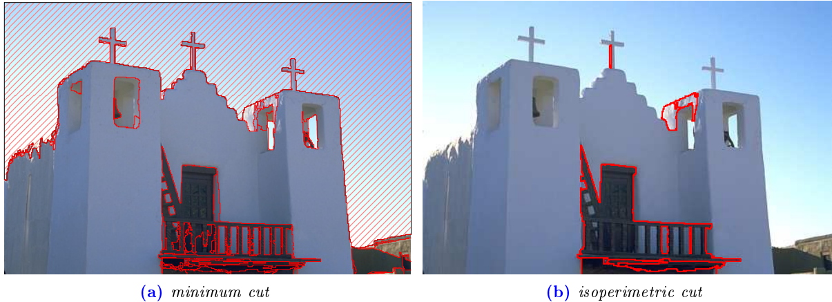
Figure 4.6: Example for isolated vertex problem. Both segmentations have been generated with mean shift as initial segmentation step. The minimum cut successfully segments the big segment (hatched on the left image).
