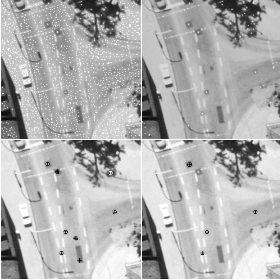
Figure 5: Results on a 170 by 170 pixels subimage using landmarks 5, 7, and 9 for learning: 2202 local maxima (top, left); 75 candidates remaining after template matching (top, right); 30 candidates with low initial error (bottom, left); 5 accepted landmarks (bottom, right).
