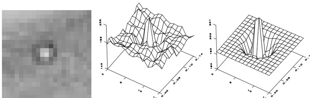
Figure 4: Intensities of landmark 7 (left, center) and of the fitted model function (right).
