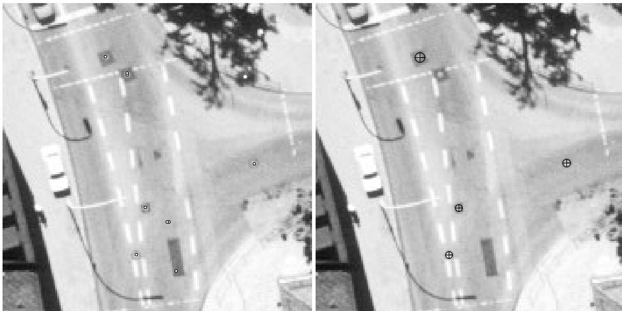
Figure 3: Results of the landmark extraction scheme applied to a small sub-image which shows five manhole covers. On the left side, small circles indicate the potential landmarks detected by normalized cross-correlation. In the final result (right) the cross centers correspond to the estimated landmark centers while the radii of the circles correspond to the values of r_{min} . Note, that one of the visible landmarks has been rejected by the verification procedure due to its high approximation error.
