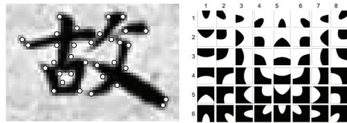
Figure 1. Interest points determined for a Chinese character using the HC detector (left). 48 templates used for classifying interest points (right).
