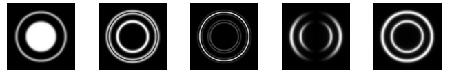
Figure 2: Left to right: original image (circular step and roof edges); gradient magnitude; squared Laplacian; oriented quadrature filter; boundary energy. Only the boundary energy yields a rotational invariant unimodal response for both step and roof edges. Filtering is done in the Fourier domain throughout the paper.
