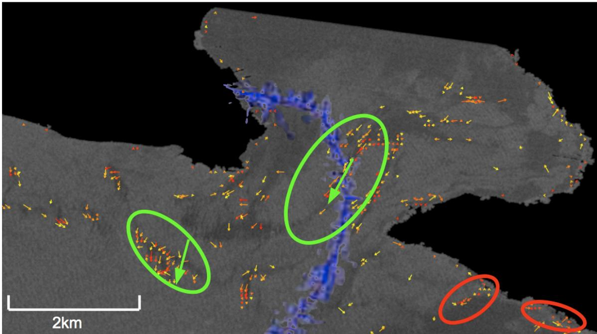
*Figure 5: A subset of the ortho-rectified and co-registered RADARSAT-2 scene with overlays. Color coded arrows of the correlation coefficient (yellow: 0.5 to red: 1.0) denote matching results of the fast NCC, blue arrows represent the in-situ measurement of the sea surface current carried out by researchers of IKI.*
