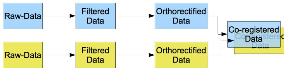
Figure 1: The developed generic pre-processing chain: According to different sensors, an individual filtering (sensor normalization) is done. Using the geometry metadata the images are automatically orthorectified. The last step, the co-registration has to be done manually. Previews are automatically generated at each step of the process chain.
