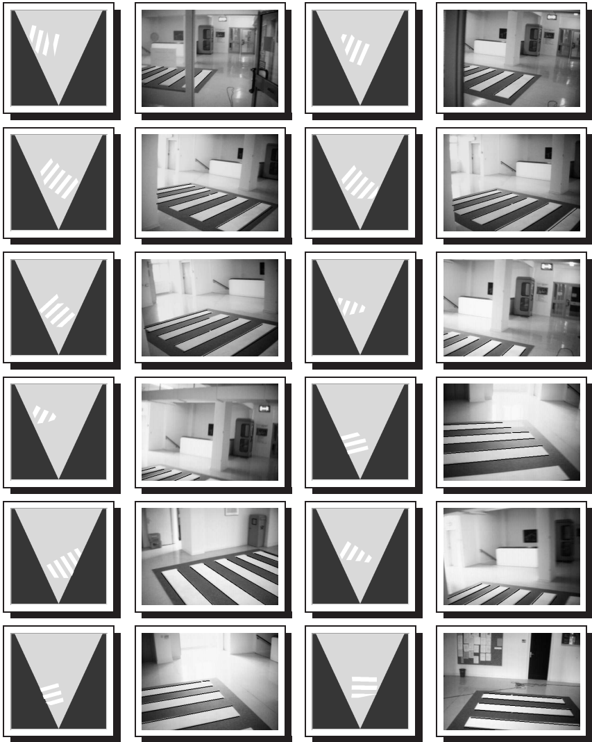
Figure 5.16: Examples of recognised zebra crossings in indoor-scenes. To the left of each image you can see a simulated birds-eye view.
