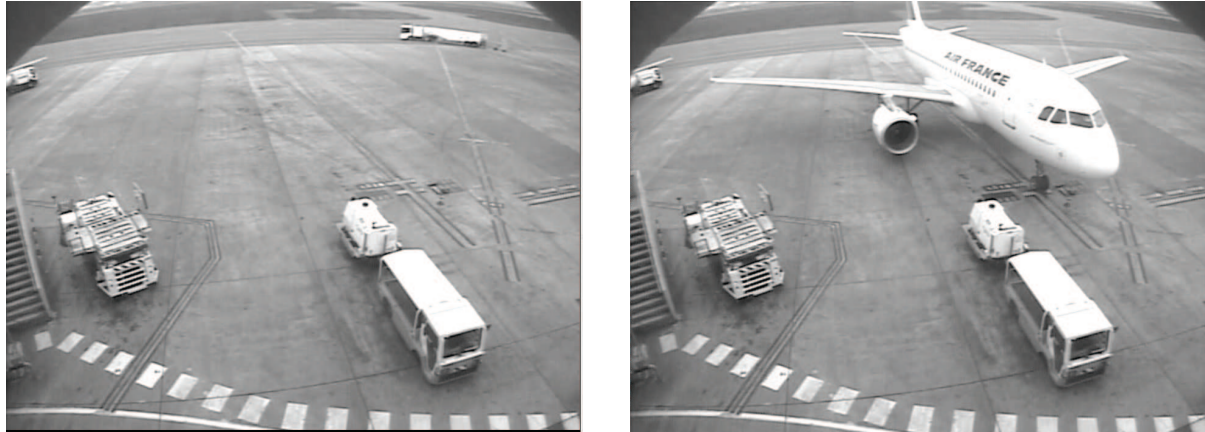
Fig. 8: Snapshots of the ERA (Entrance Restricted Area) after completing Arrival-Preparation . The GPU (Ground Power Unit) and chocks are in place. The tanker crossing the ERA in the background (left) causes an erroneous interpretation thread (see text).
