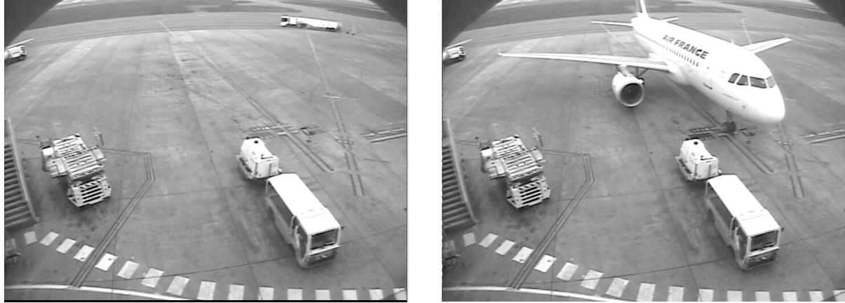
Fig. 16: Snapshots of the ERA (Entrance Restricted Area) after completing Arrival-Preparation . The GPU (Ground Power Unit) and chocks are in place. The tanker crossing the ERA in the background (left) causes an erroneous interpretation thread (see text).
