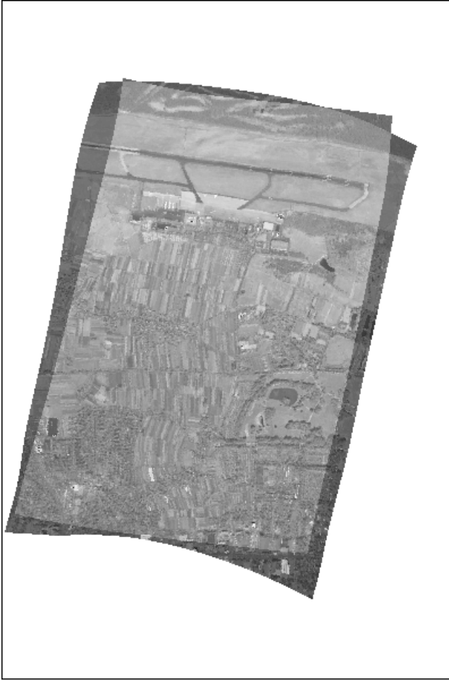
Figure 3: Overlay (addition and rescaling) of the two map-registered images of 1991 and 1995 (using thin-plate spline registration with U(r) = r^2 \ln r ).
