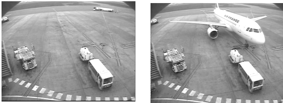
Figure 6. Snapshots of the ERA (Entrance Restricted Area) after completing Arrival-Preparation . The GPU (Ground Power Unit) and shocks are in place. The tanker crossing the ERA in the background (left) causes an erroneous interpretation thread (see text).
