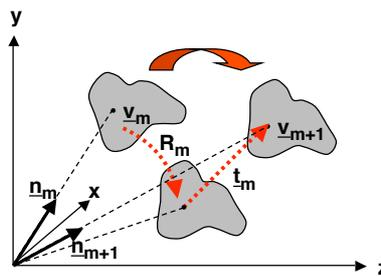
$R_m \underline{n}_m$ ,  $\underline{t}_m$  and  $\underline{n}_m$  are coplanar:  $[\underline{t}_m \times R_m \underline{n}_m]^T \underline{n}_{m+1} = 0$
