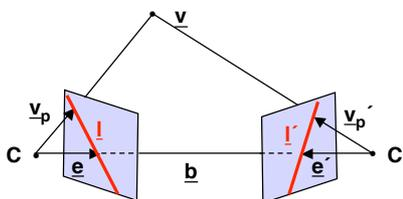
The epipoles  $\underline{e}$  and  $\underline{e'}$  are the intersection points of the baseline with the image planes. The epipolar line  $\underline{l}$  and  $\underline{l'}$  mark the intersections of the epipolar plane in the left and right image, respectively.
