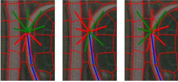
Figure 2. Results of the sub cost functions  $c_{angle}$ ,  $c_{border}$ ,  $c_{region}$  (l.t.r.) of the overall cost function  $c$ . Red: continuation not possible. Green: continuation possible. Image source: Google Earth, Copyright by Google Inc.
