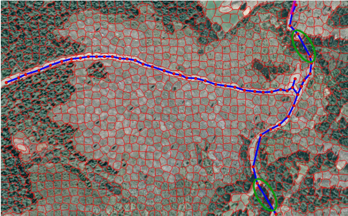
Figure 3. Result of the proposed road tracker. Seed is marked in pink (top right). Multiple occluded parts of the road (green) as well as a junction are correctly tracked. Image source: Google Earth, Copyright by Google Inc.
