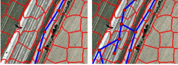
Figure 4. Effects of the use of the border ( $c_{border}$ ) on the results of the proposed road tracking algorithm. Left: border is used. Right: border is not used. Image source: Google Earth, Copyright by Google Inc.
