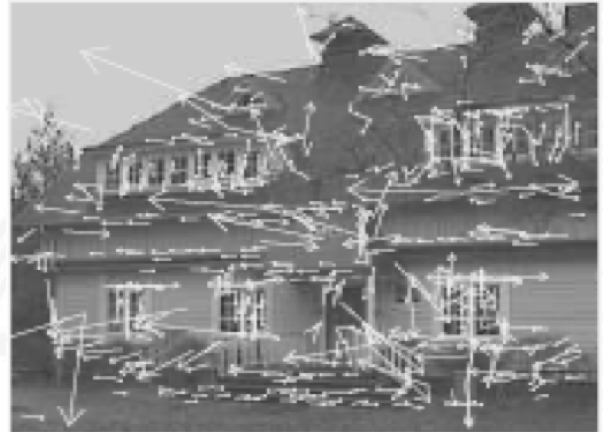
536 keypoints remain after applying threshold on ratio of principal curvatures
