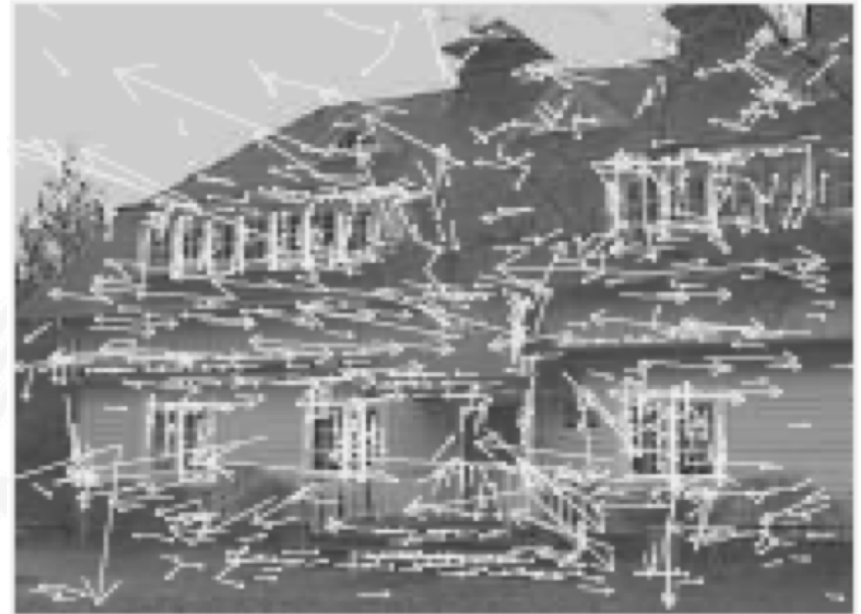
832 keypoint candidates at extrema of DoG images. Vectors show location, orientation and scale.
