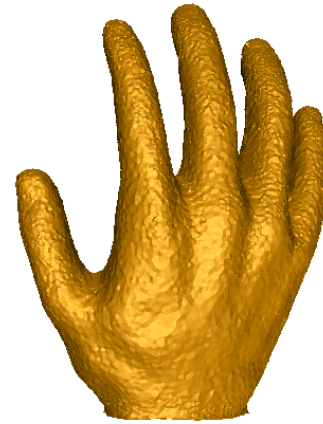
Figure 10. To demonstrate robustness in the presence of noise, we added Gaussian noise to laser range scanner data. The resulting model is still watertight.
