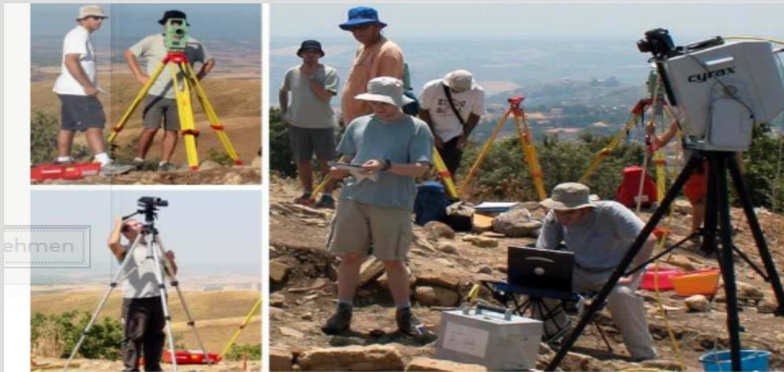
**Figure 1.** Members of our team record exact 3D coordinates using a total station surveying instrument (upper left), capture video of an excavation using a scanner and digital camera (lower left), and scan a portion of the excavation site using a time-of-flight laser range scanner (right).
