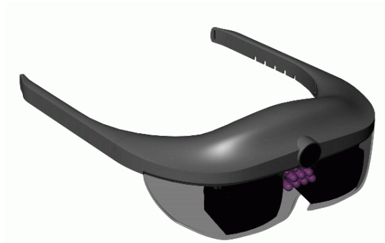
Figure 5: A spectacle-like night-vision system for persons with night-blindness, developed by partner 5.
