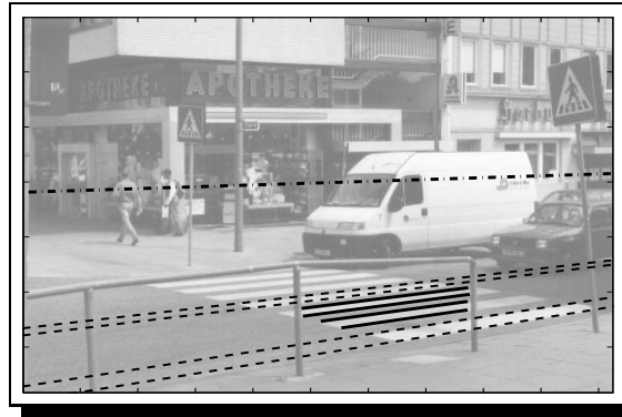
Figure 5.4: Grouping zebra crossings zebra-crossings . Starting with a set of 4 coincident line segments line-segments (continuous lines), a vanishing line vanishing-line (dot-dashed line) is calculated and additional lines corresponding to adjacent stripes are hypothesised (dashed lines).
